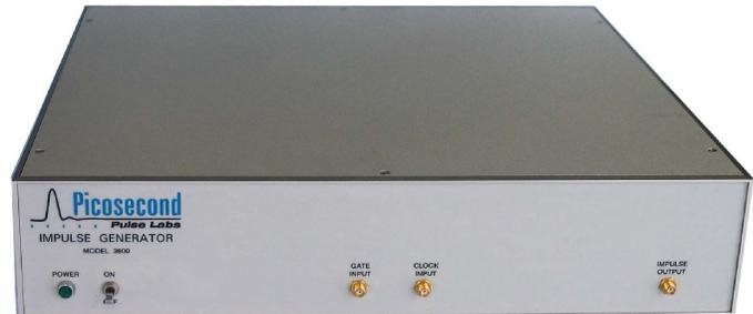
The Model 3600 Impulse Generator produces 7.5-volt, 70 ps duration impulses that are locked to a clock or sine wave input. The added jitter is less than 2 ps. The impulse train can be gated by an external TTL signal. The Model 3600 will function at repetition rates ranging from < 100 Hz to 2.5 GHz.
